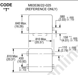
All Enclosures have cupro-Nickel cans bright acid tin/lead plated after assembly to terminal headers.
