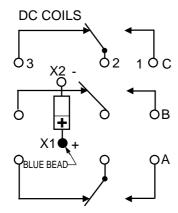
**NOTE:** Polarity must be observed with DC coil supply. Relay is polarized with a permanent magnet and will not operate or be damaged by reverse polarity.
