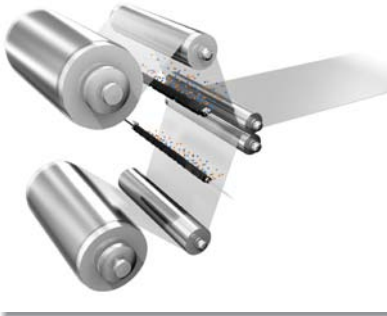
Removing dust while separating TAB protective film
