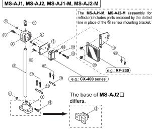
Note: The assembly for reflector (**MS-AJ-M**) does not contain the **(6)** cable quide
