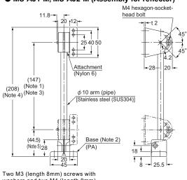
washers and two M4 (length 8mm) screws with washers are attached.
