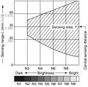
The shaded area shown in the figure at left indicates the sensing range. Be sure to set up the sensor with enough margin – the sensing range may vary from unit to unit.
