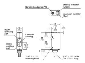
(\*1): The **UZD60** is not incorporated with it. It is substituted with the timer adjuster on the **UZD621**.
