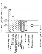
The bar graph on the left indicates the sensing range. Be sure to set up the sensor with enough margin – the sensing range may vary from unit to unit.
