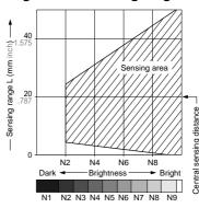
The shaded area shown in the figure at left indicates the sensing range. Be sure to set up the sensor with enough margin – the sensing range may vary from unit to unit.
