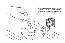
Note: Do not expose it to water splash during operation. If it may so, it detects water drop on it.
