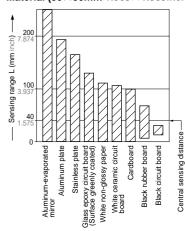
The bar graph on the left indicates the sensing range. Be sure to set up the sensor with enough margin – the sensing range may vary from unit to unit.
