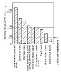
The bar graph on the left indicates the sensing range. Be sure to set up the sensor with enough margin – the sensing range may vary from unit to unit.
