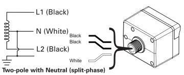
120V (L-N) / 240V (L1-L2), single-phase (split) center tap For installations at or less than 10 feet (3m) from the transformer. Catalog number: SPP40SP2240PN
