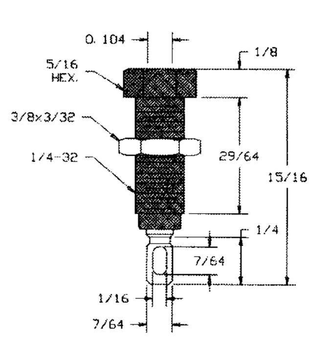
Part is completely insulated from chassis. Accommodates panels from 1/16" to 1/4" thick. Design of part accepts miniature banana plugs. One piece turret contact allows sealed panel entry hole.
