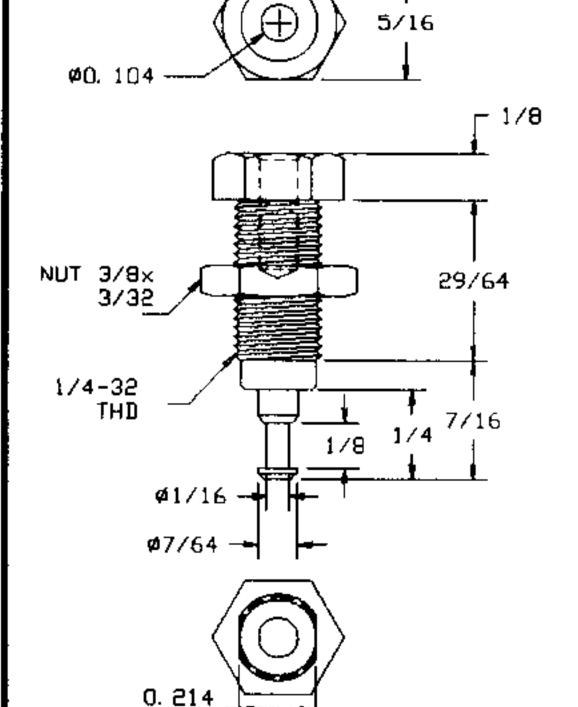
Part is completely insulated from chassis. Accommodates panels from 1/16" to 1/4" thick. Design of part accepts miniature banana plug. One piece turret contact allows sealed panel entry hole.
