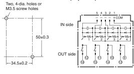
Note: Do not reverse the coil polarity.
