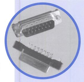
The Amphenol "TF" series features eye of needle formed contacts, and insulator with closed entry contacts cavities.
