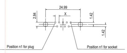
For PCB holes diameters, see on page 1 (finished holes)
