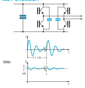
L = stray inductance IGBT + capacitor R = serial resistance IGBT + capacitor
