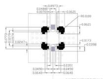
$2 \times \text{TRANSMISSION LINES 50 } \Omega$ Dimensions are in mm (inches)
