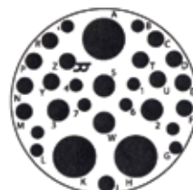
25-20 - 25-20* 3 #8 Twinax, 13 #16, 4 #12 Coax, 10 #20 N / Coax / Twinax
