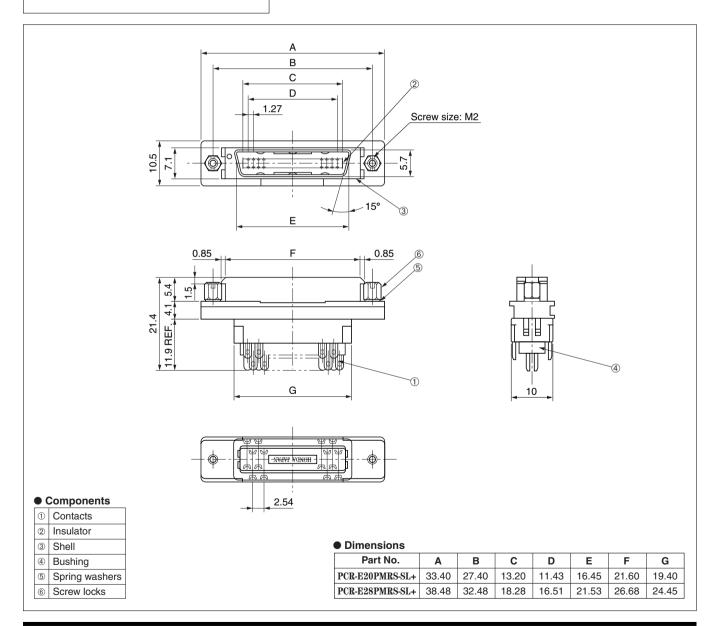
Mating connectors: PCR series cable-side IDC type or soldering type female connector
