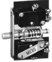
AC Series Door Switch, Single Pole Double Throw Double Break Circuitry, 15 A at 250 Vac, Steel Rod Actuator, Screw Termination
