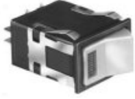
AML34 Series Rocker Switch, SPST, 2 position, Silver Contacts, 0.187 in x 0.02 in (Solder or Quick-Connect), Non-Lighted, Rectangle, Snap-in Panel
