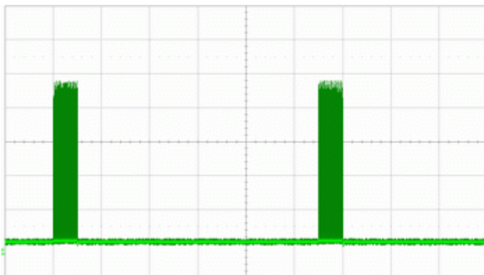
Locked rotor current @ 48 V ( I = 200\text{mA/div} ; t = 1\text{s/div} )
