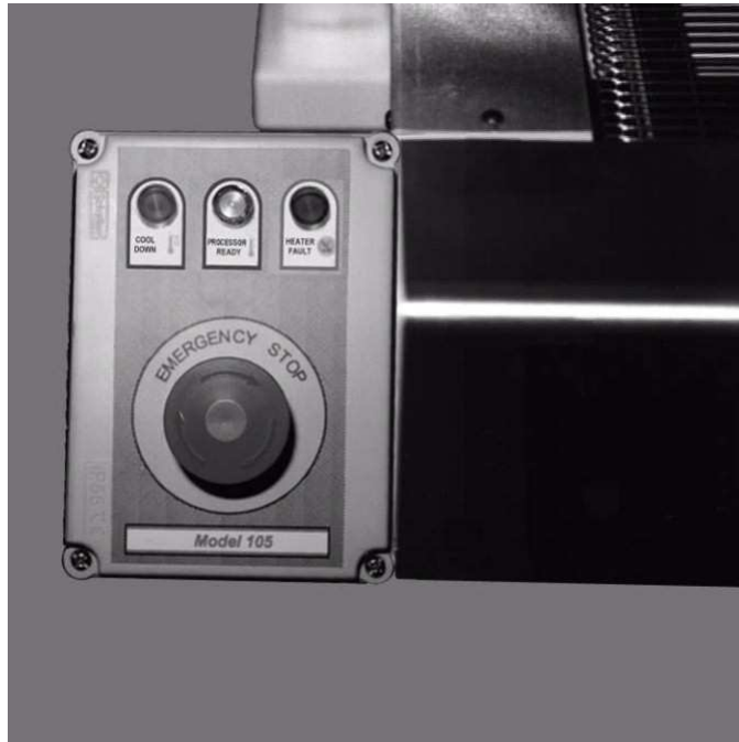
Emergency Stop Enclosure
